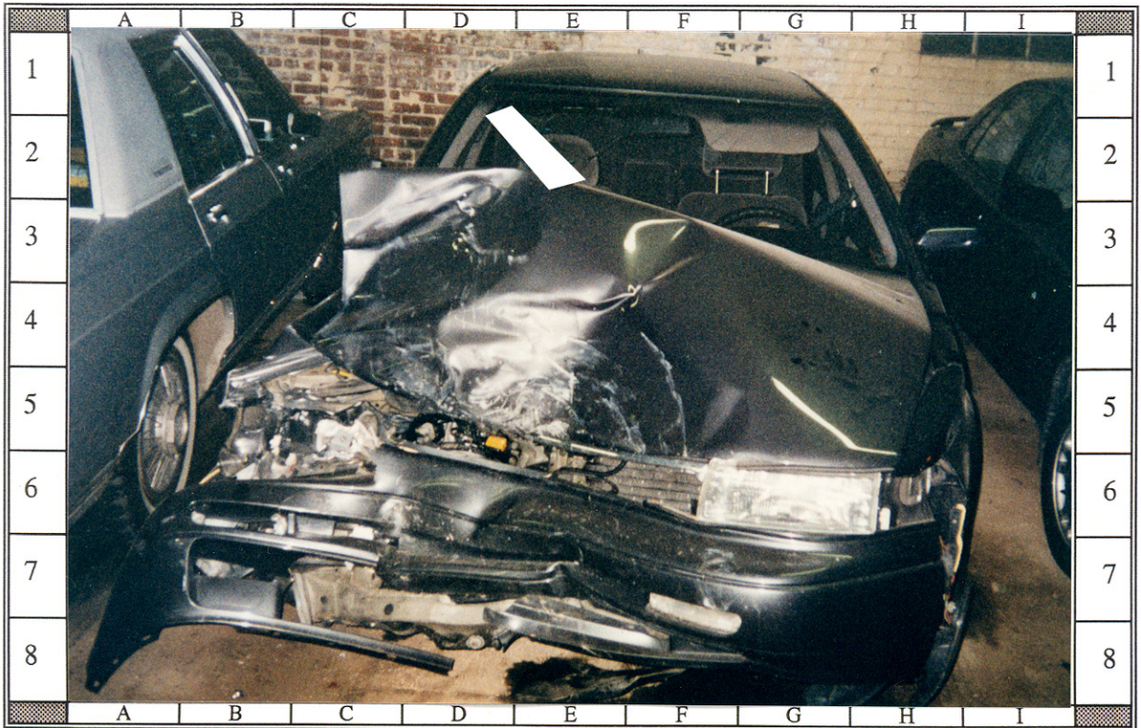
# 09: Case Vehicle's direct frontal damage showing offset nature of impact to vehicle's front right half; NOTE: two-point motorized shoulder belt is connected to track
